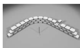
Inside curves increase in radius towards the top of the wall.
