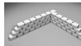
Use full blocks in the corner of inside corners.
