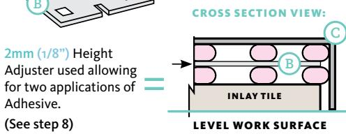
**NOTE NUMBER OF KEYWAYS REQUIRED:** 10, 20 & 30mm (0.4", 0.8", & 1.2") lids require one keyway cut and 40, 50 & 60mm (1.6", 2", & 2.5") lids require two keyways cut at opposite ends of the stone to suit inlay lid.
