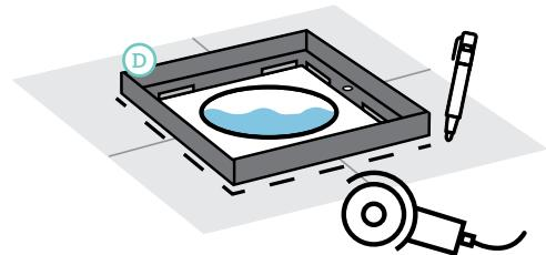
**⚠** Ensure edge protector is centred over skimmer to mark cutting area. Allow for 1-2mm (1/16") clearance on all sides.
