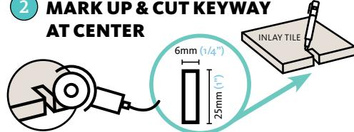
Ensure keyway is positioned on the tile edge which will be closest to the pool. Check that the key fits the keyway before gluing.
