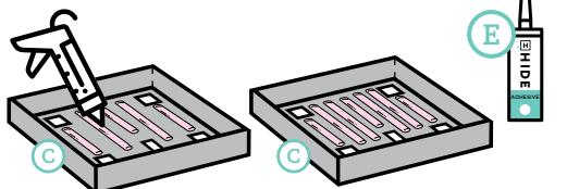
**⚠** Avoid placing adhesive within 10mm (3/8") of keyway and drainage holes.
