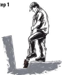
**Step 1** - Dig a shallow trench, level and place 100mm of crushed rock in the bottom. Level and compact. Allow for 50mm embedment of the bottom course and 300mm behind the wall for drainage.
