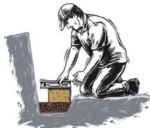
**Step 2** - Spread and level approximately 25mm of coarse sand as a bedding layer then place the first course of Versawall™ units. Use a stringline for creating a straight line, and level from side to side and front to back. Install a 90mm Agricultural Pipe (on grade) at the rear of the wall for drainage.
